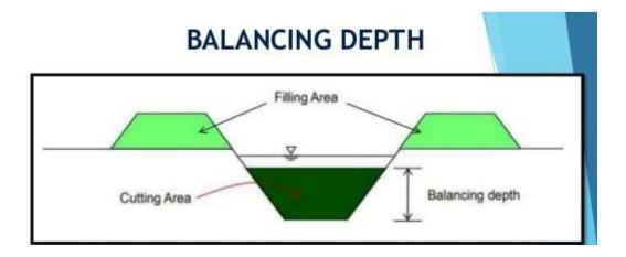
If for a channel section the depth of cutting is such that the quantity of excavation or cutting is equal to the earth filling required for making the banks, then depth of cutting is known as balancing depth or most economical depth of cutting.
